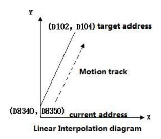
In the Center interpolation: D100 is speed, D102 is the X-axis target address, D104 is the Y-axis target address, and D106 is the center X address. D108 is the center Y address. Y0 and Y1 respectively pulse the X-axis and Y-axis.
