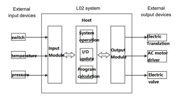
Above is a simple expression of the operation of the host, which simplifies the process of initialization, diagnosis, communication and other system aspects, and the process of external interruption, time interruption and other
