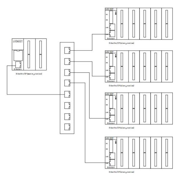
2. The L02 host is the master station of the Ethernet/IP protocol, and the L02-EIP is the slave station of the Ethernet/IP protocol, without going through the router.
