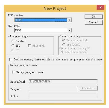
Select in the GX Works2 software version as shown in the figure: (Note: the use of labels is prohibited)
