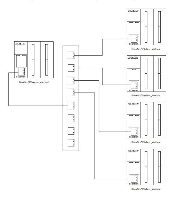
4. The L02 host is the master station of the Ethernet/IP protocol, and the L02 host and the L02-EIP module are mixed as the slave station of the Ethernet/IP protocol
