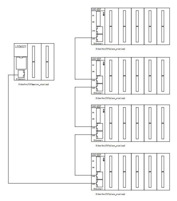
3. The L02 host is the master station of the Ethernet/IP protocol, and the L02 host is the slave station of the Ethernet/IP protocol.
